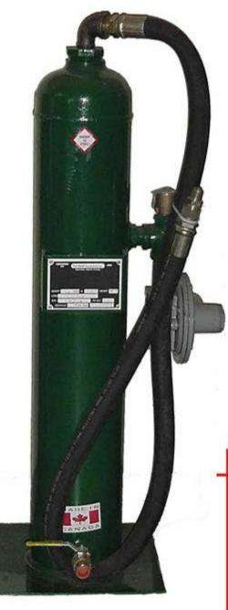
Application: SVT - A Propane SVT - B Casing / Natural Gas SVT - A No High Level Shut Down (HLSD) Valve SVT - B HLSD included MAWP: 12 psig (non-coded vessel) Inlet/ Outlet: 1" NPT Max Inlet Pressure: 60 psig Regulator Outlet Pressure: 4 - 9 " W.C. Standard -----6 - 16 " W.C. Hose: 1" x 6' - with 1/2" J.I.C. Connector
